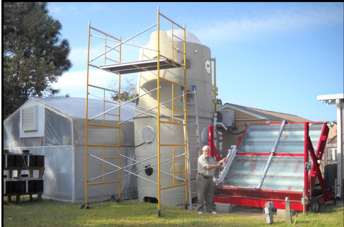
8' X 15' round bioreactor with a 8' X 8' flat panel photo-bioreactor unit adjacent to the outdoor greenhouse and laboratory facility. Total volume @ 4500 gallons (18,000-liters)
